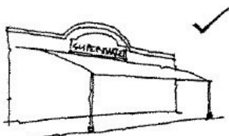
Panels should not intrude into the skyline when viewed from the street.
